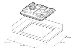
NOTE: Distances shown to adjacent walls/surfaces are for the distance to a combustible surface. If the surface is not combustible the measurement
