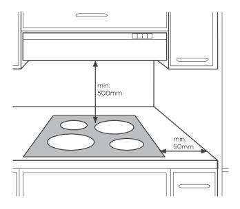
NOTE: The clearance must meet or exceed the minimum recommended for both the rangehood and cooktop. Refer to the rangehood installation manual.
