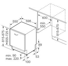
measurements in mm
