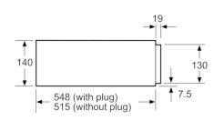
Compact ovens with an appliance height of 455 mm can be installed above a warming drawer. An intermediate floor is not required.
